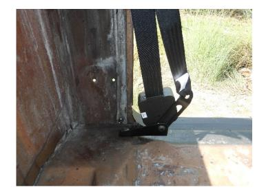
8. Once you have the retractors mounted and the shoulder loop installed you can bolt in the buckles.
